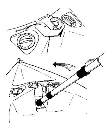
$\checkmark$  Push the boom jaws onto the *mast* just <u>above</u> the mast collar until they snap in place.
