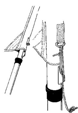
✓ Lay the *daggerboard* in the boat close to the *mast* and leave it there until the boat has been launched.
