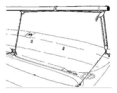
✓ Attach the *vang* to the *mast* by clipping the snap hook to the eyestrap just above the *mast gate*. Leave the *vang* adjustment very loose and after the *mainsail* is rigged adjust and cleat the *vang* so the *boom* will be no more than slightly above horizontal while sailing.
