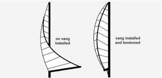
In a seaway, your boom will bounce around. That's tough on the boom and boom fittings. And the mainsail leech? It'll belly out like a pregnant whale--dumping lots of wind (above left). Your boat will be tough to control as weather helm increases.
