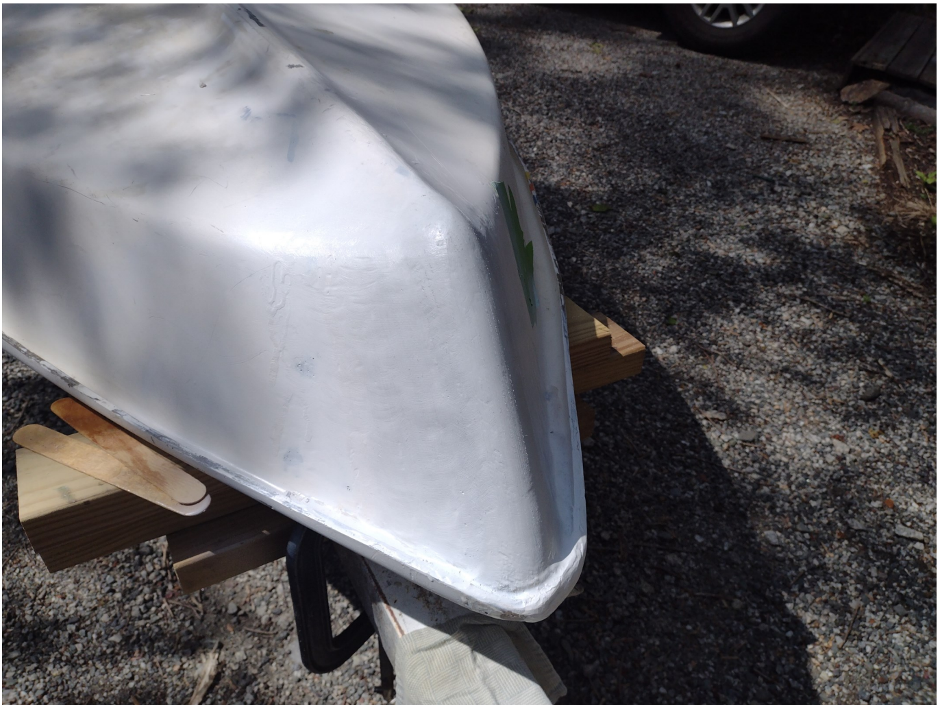
04 5plies of mat, fairing tape applied
