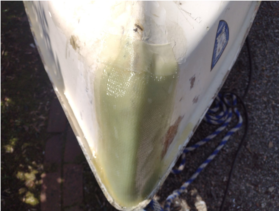
04 5plies of mat, fairing tape applied
