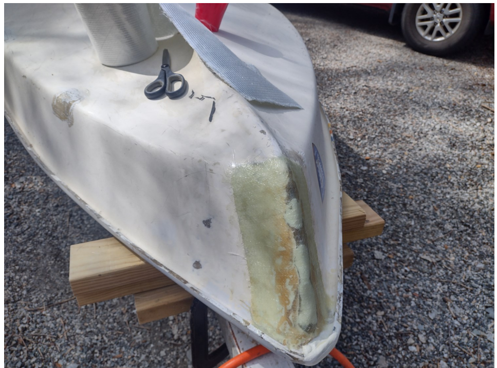
03 First ply of fiberglass mat applied
