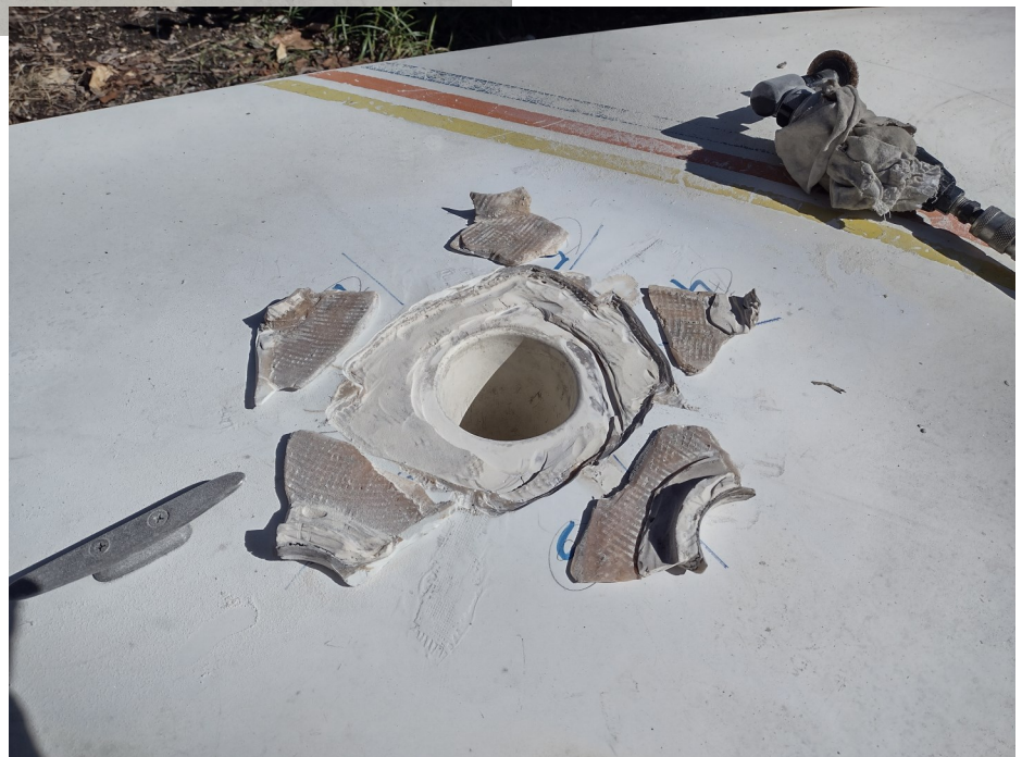
02b Broken pieces cleaned and smoothed
